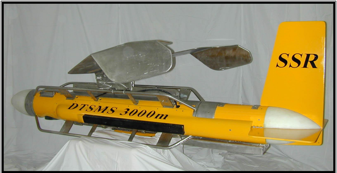
SSR's DTSMS 3000m rated Deeptow System with Depressor Wing
